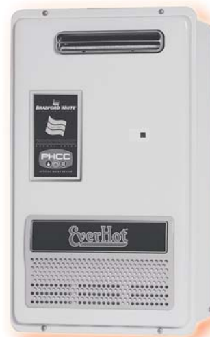
The Bradford White Everhot tankless water heater is available with outputs of 3.87 and 4.26 gpm and is designed to be manifolded with multiple units for larger water quantities.
